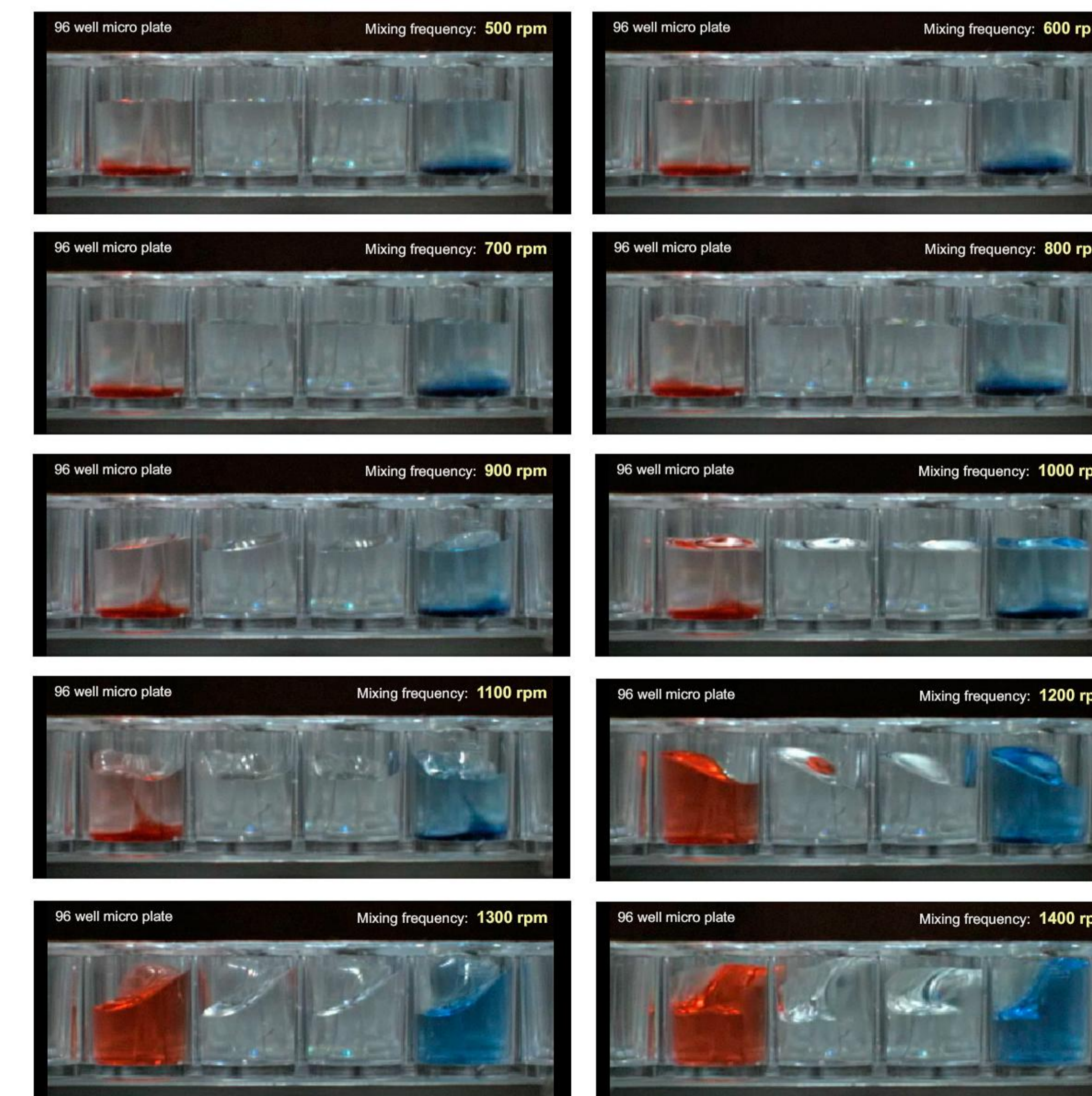
Figure 3: Experimental studies of the mixing behavior in a 96 well plate depend on preselected mixing speeds. For aqueous solutions with 210 \mu l filling volume/well the ideal shaking frequency should amount 1,200 rpm. Below 1,000 rpm, only inadequate mixing results can be reached in a short time. From 1,400 rpm start of the danger zone of possible spilling effects of the samples.
