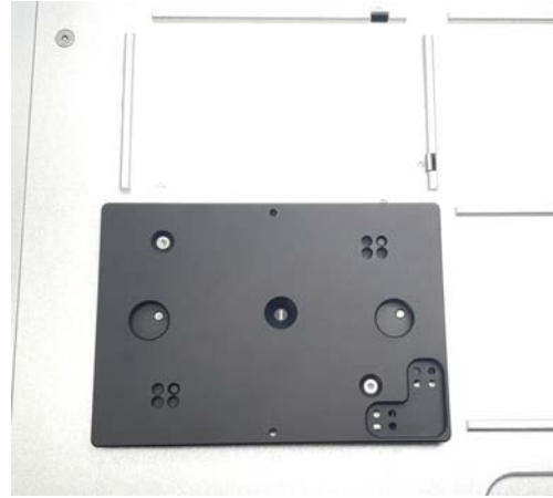
Figure 13 View of the OT-2 deck with the QOT plate mounted at deck position 1 with set-up number 1 using the mount option C
