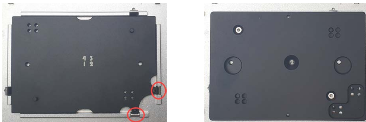
Figure 5 The image on the left only shows the OT-2 plate for visualization and understanding reasons. The OT-2 plate is hold in position by the two leaf springs in the right lower corner of the OT-2 deck (red circle). The image on the right shows the complete QOT plate placed at deck position 3, with set-up number 2
