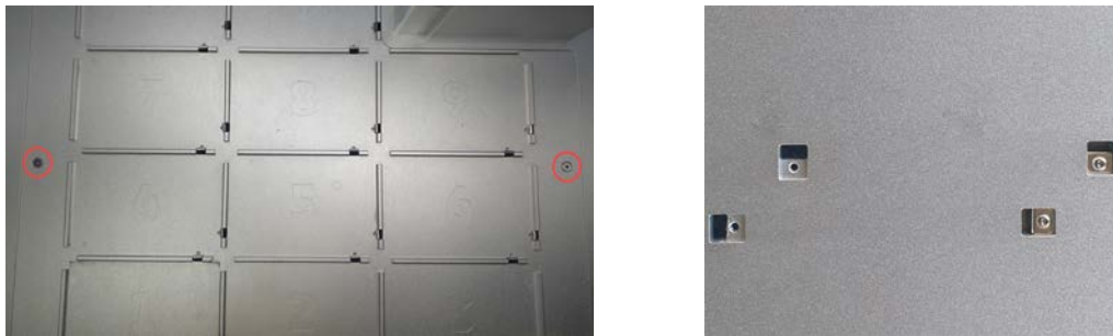
Figure 6 Image on the left shows of the OT-2 deck with red circles around the screws holding the deck plate. Image on the right shows the bottom-side of the OT-2 deck plate, with removed (left) and not removed (right) leaf springs.
