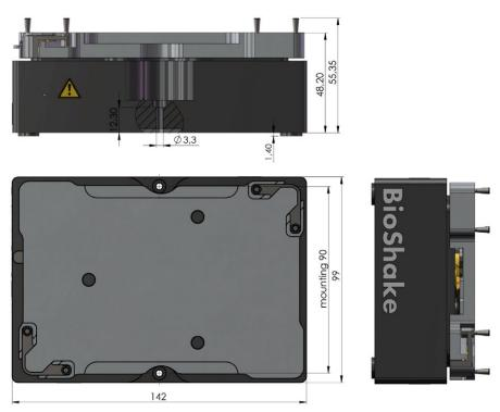
Figure 1 Technical drawing of device
