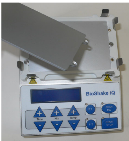
Removing of security cover (step 4)
