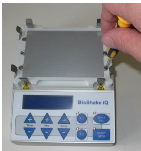
Loosen the 3 screws (step 3)
