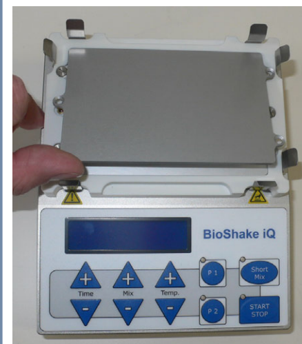
Step 4: Lift up of security cover (step 4)
