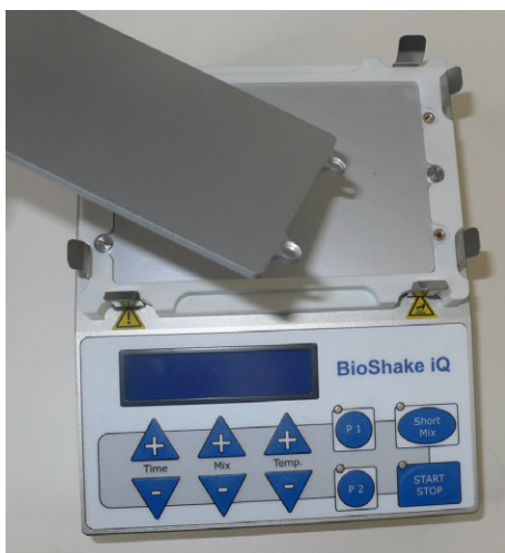
Removing of security cover (step 4)
